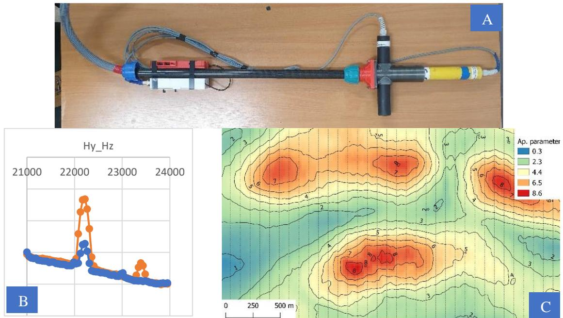
**Figure 1** SibGIS UAS VLF system (a); sample of FFT result: amplitudes of horizontal ( $H_y$ ) and vertical ( $H_z$ ) components of EM field at 22.2 kHz frequency (b); sample of map of apparent parameter (c)
