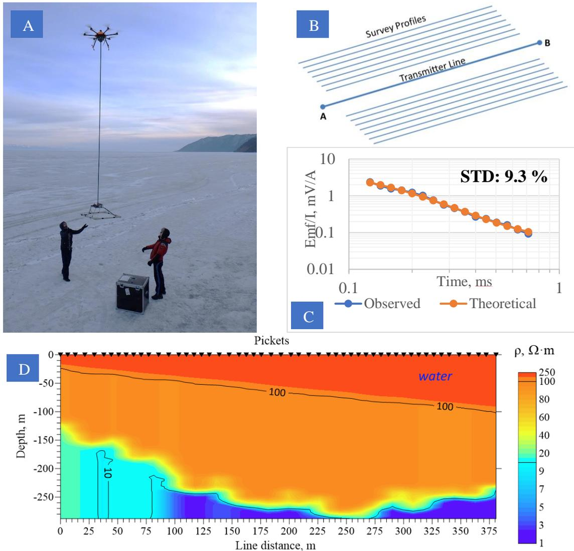
**Figure 2.** SibGIS UAS-TEM system: at flight (a), geometry of measurements (b); samples of obtained and model sounding curves(c); and example of 1D inversion (d).
